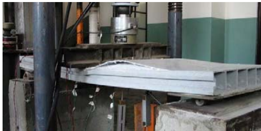
Fig. 3: Failure of GFRP deck
