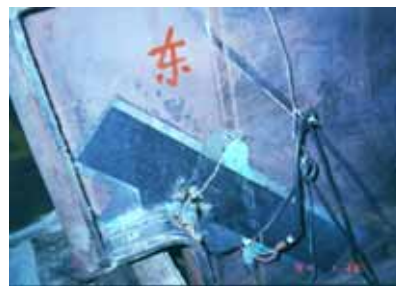
Figure 11 Fatigue test of steel beam strengthened with CFRP at the support
