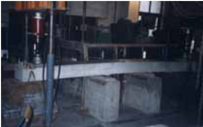
Figure 1 Test of RC bridge slab strengthened with CFRP sheets under
