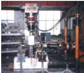
Figure 2 Test set of RC column strengthened with CFRP sheets
