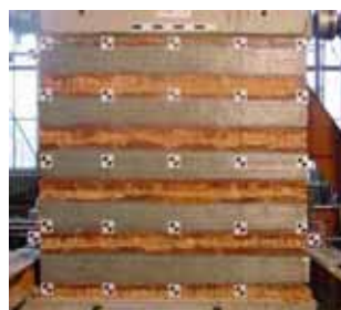
Figure 13 Masonry wall strengthened with GFRP
