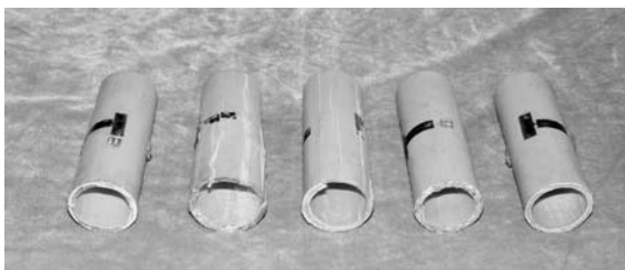
Fig. 2 Failure mode of short GFRP pipes
